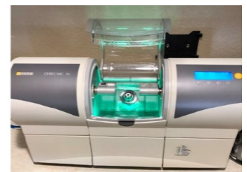
The milling machine used to make crowns using CAD/CAM technology.
